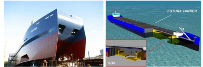
Figure 11. Typical bow section of a FUTURA TANKER (left), impression of the SOS integrated into a FUTURA TANKER (right)
