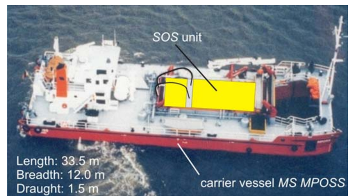
Figure 3. Schematical illustration of MPOSS with integrated SOS unit
